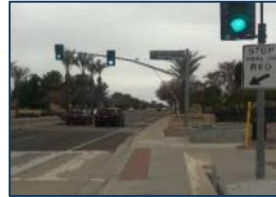
Signalized mid-block crossing: signal between roadway intersections
