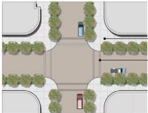
Scored and or Colored Concrete Within Sidewalks at Intersections Typical Striping at Crosswalks
