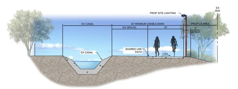
HIGHLINE CANAL SHARED USE PATH EXTENSION TYPICAL SECTION (LOOKING NORTH)
