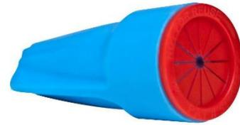
Commercial irrigation systems use a different type of connector, commonly referred to as Dri-Splice or Pentite connectors. These are preferred as they must be cut off when replaced and they cannot be re-used. This makes it necessary to install a new connector whenever a repair is done.
