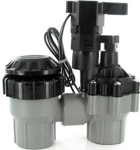
Your system may be using a different type of backflow preventer, they are called anti-siphon valves. Each valve has a type of backflow preventer built in. While these are compliant with codes, they cannot be tested so they are not the preferred method. Over time the gravity operated seal can become stuck in the closed position giving a false sense of protection. These valves are also installed above ground and need to be protected from the sun and any other accidental damage.
