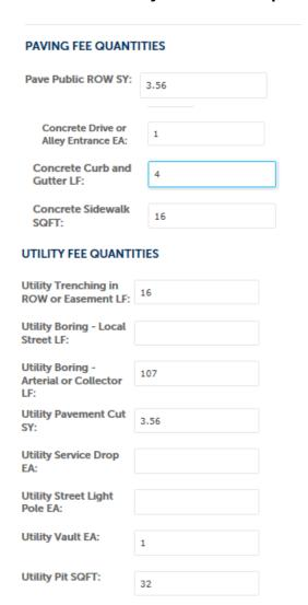
For long bores where the number of bore pits is not yet known or relief pits are going to be needed City staff will estimate a 2' wide by 4' long bore/relief pit for every 500' of boring unless those pits are shown on the plans.
