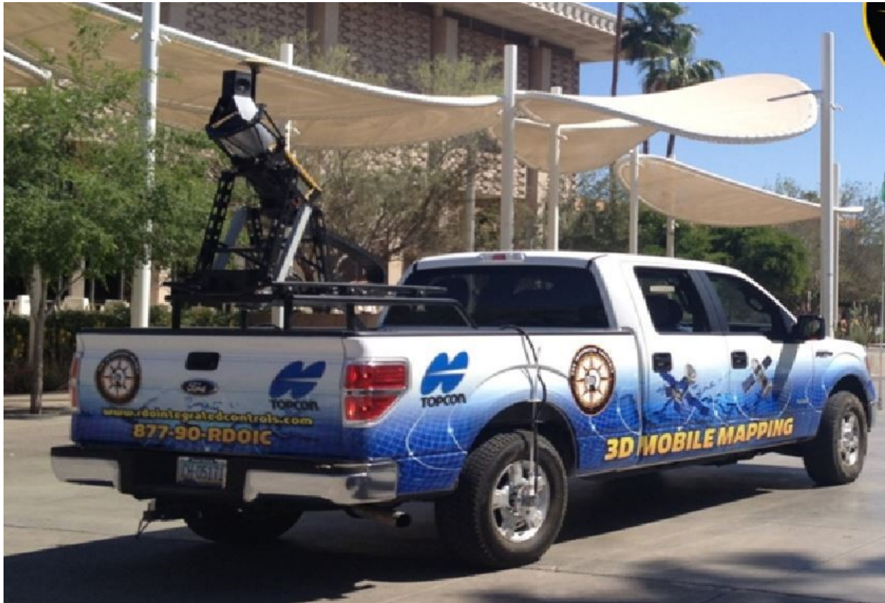
Figure 2 Mobile Mapping (LiDAR) Scanning Vehicle
